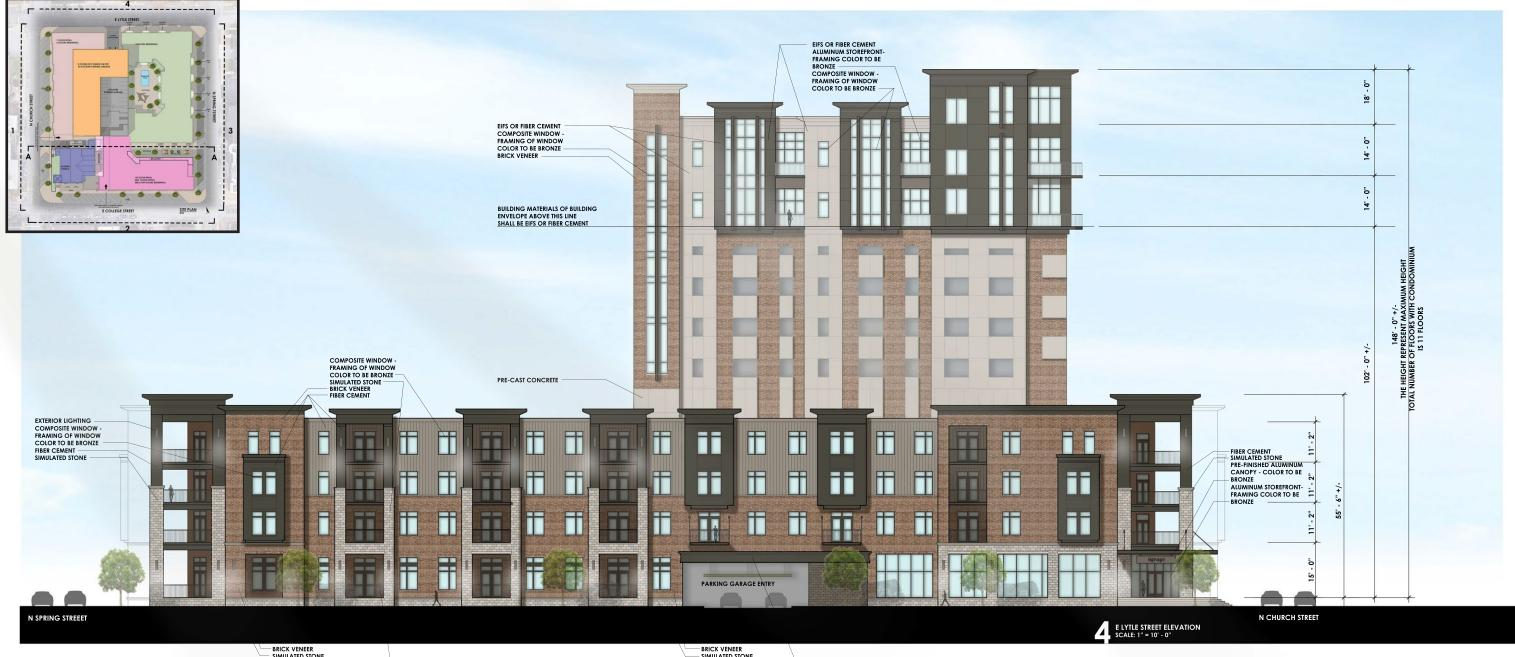
BRICK VENEER SIMULATED STONE FIBER CEMENT BANDING
