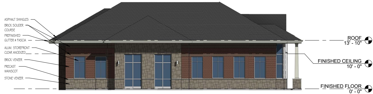
Building 4 - Office Building - South Elevation
