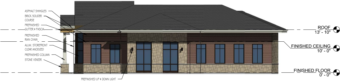
Building 3 - Office Building - South Elevation
