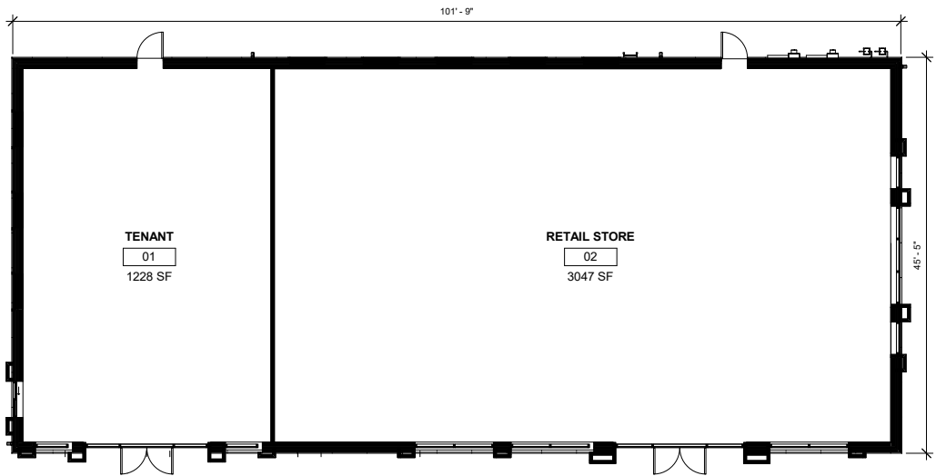
Building 1 - Gas Station with Retail - Floor Plan
