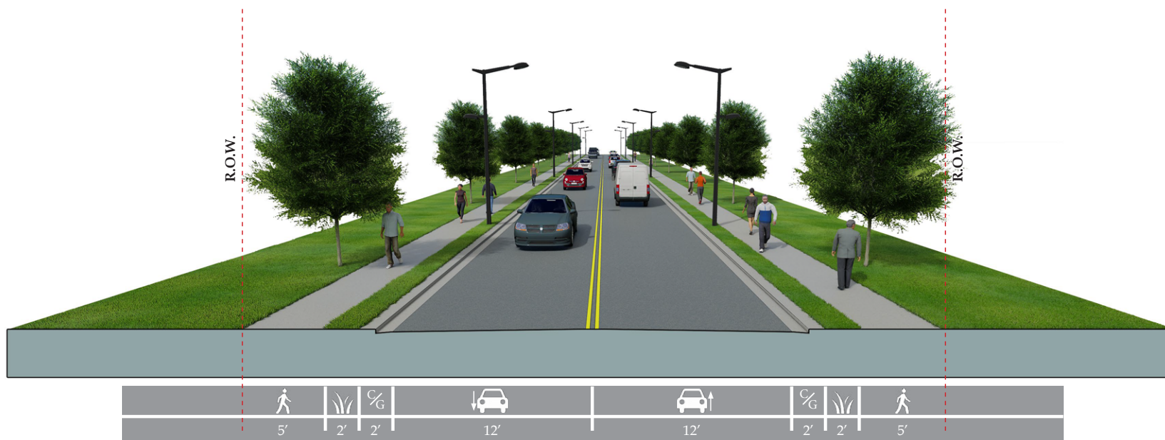
Example of 42-foot R.O.W. Cross Section
