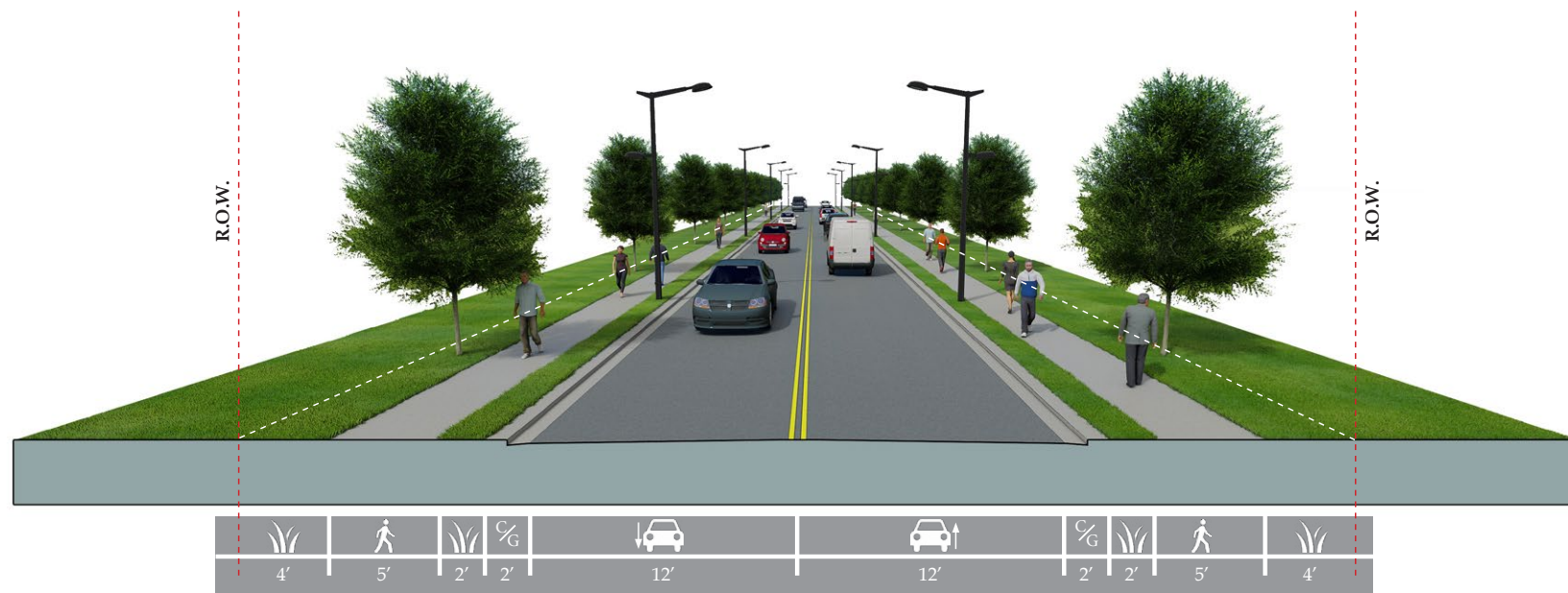
Example of 50-foot R.O.W. Cross Section
