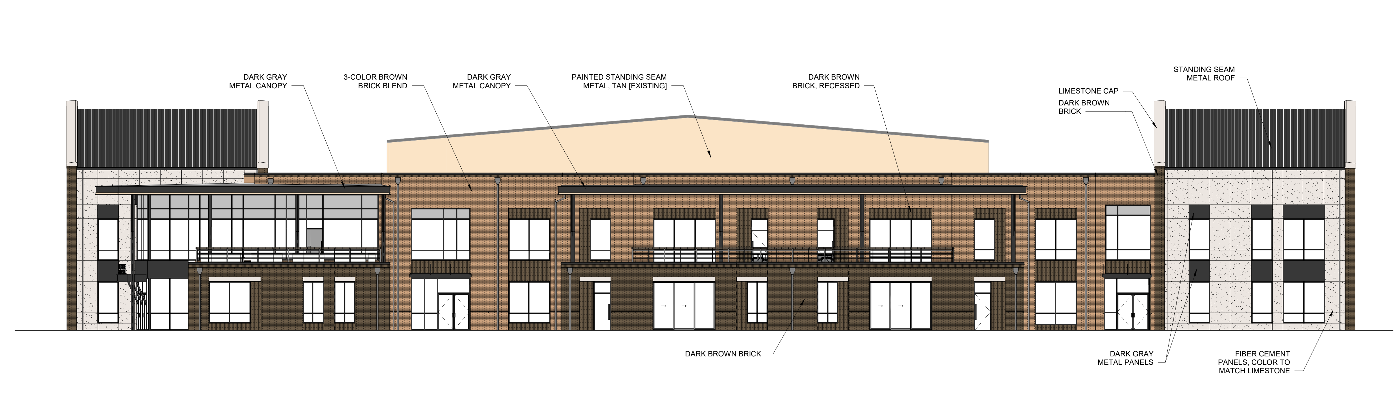
EXTERIOR ELEVATION WEST
