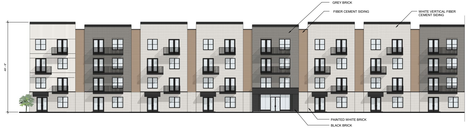
4 BUILDING D NORTH (CTYD) (TOWARDS COURTYARD)
