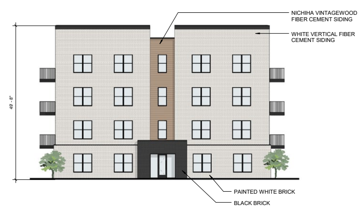
3 BUILDING D EAST ELEVATION (TOWARDS OFFICE BUILDING)
