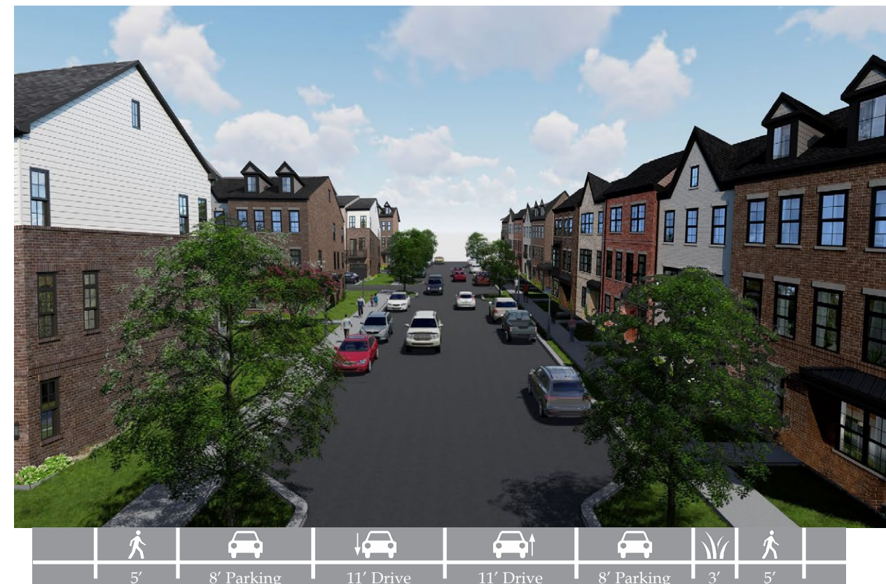
Typical 53-Foot Private Drive Cross Section
