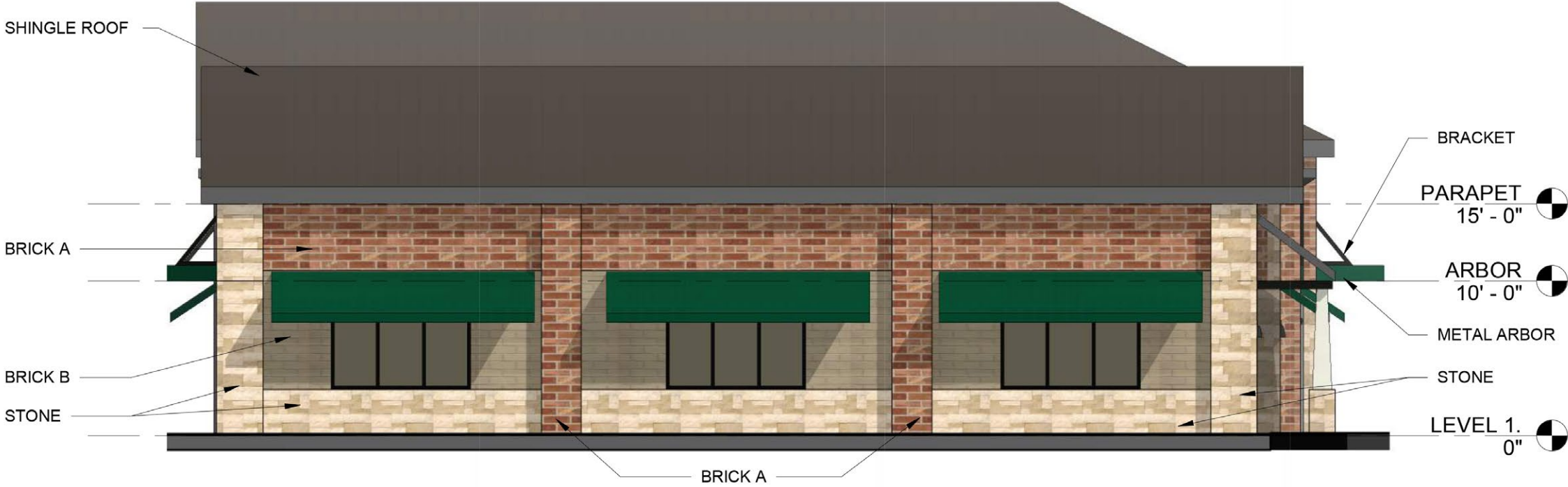
E4 SOUTH- EXTERIOR ELEVATION (Side)
