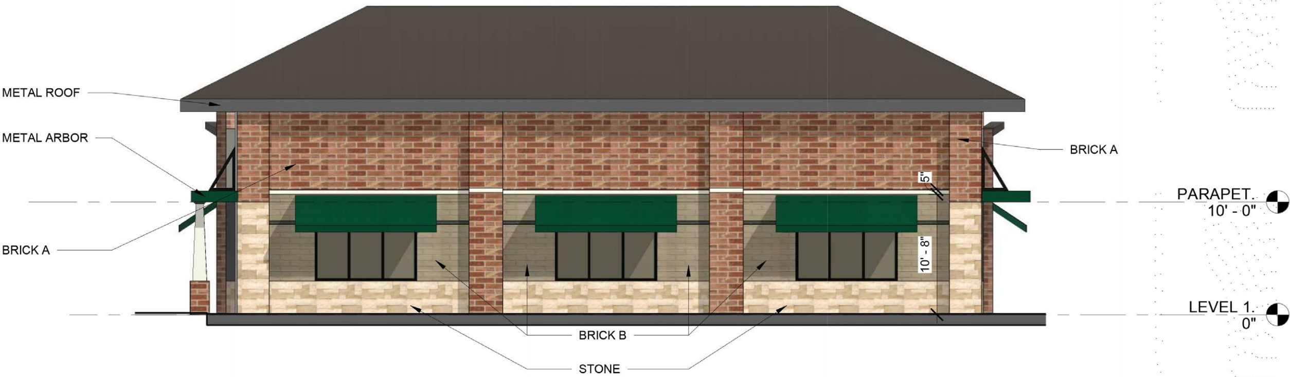
C5 EAST- EXTERIOR ELEVATION (Side)
