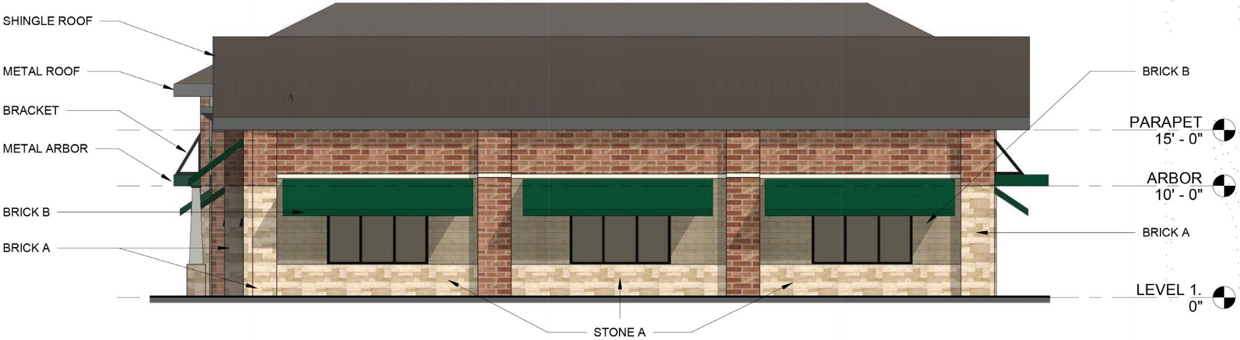
C5 SOUTH- EXTERIOR ELEVATION (Side)
