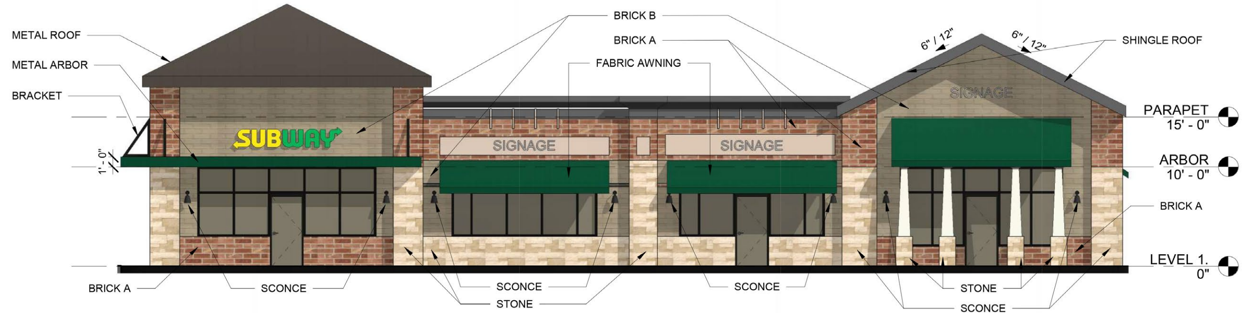
C1 WEST - EXTERIOR ELEVATION (Front)
