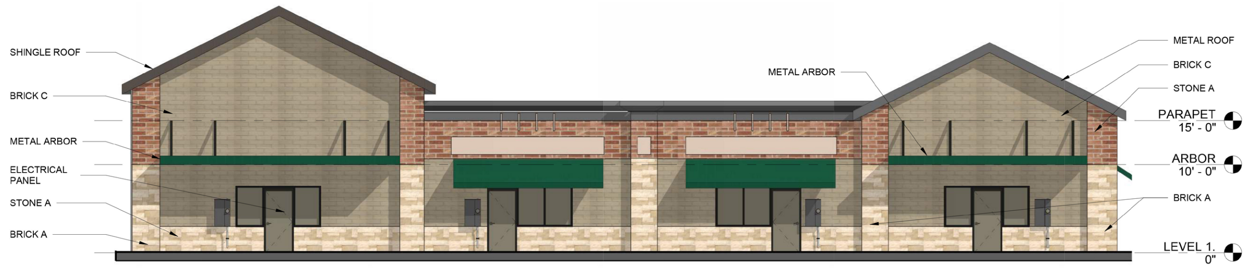
C2 EAST- EXTERIOR ELEVATION (Rear)
