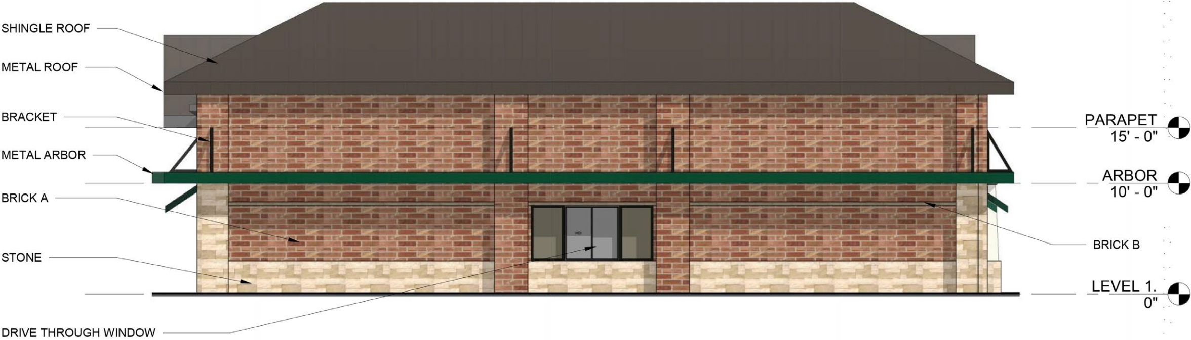
C2 NORTH-EXTERIOR ELEVATION (Side)
