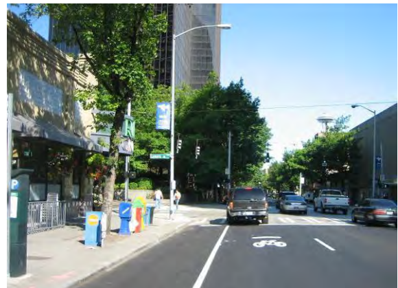
Example of the Shared Lane Pavement Marking also called a “sharrow”, 2009 Edition of the MUTCD
