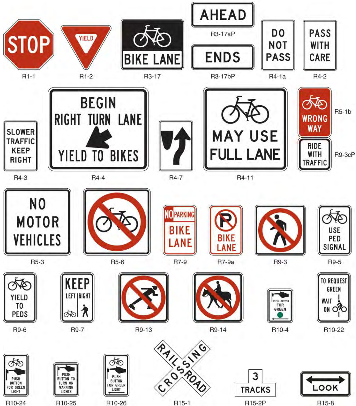
Regulatory bicycle facilities signage from the 2009 edition of the Manual on Uniform Traffic Control Devices .
