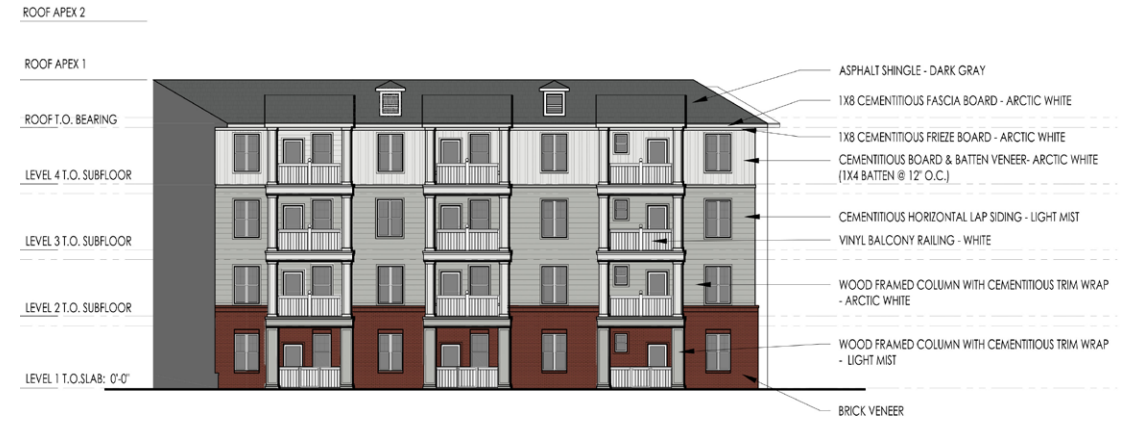
3 REAR ELEVATION (REAR LEG - RIGHT SIDE)
