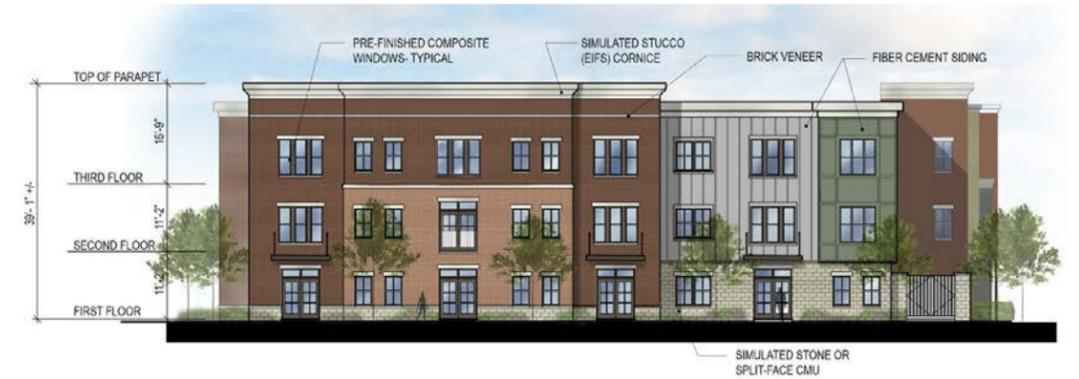
BUILDING 3 - ELEVATION C.3 (GREEN) - STATE STREET ELEVATION
