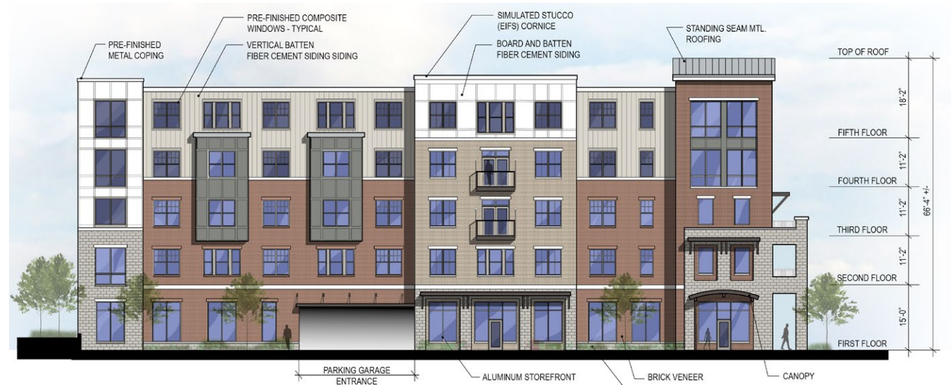
BUILDING 2 - ELEVATION B.2 (BLUE) - NORTHWEST (FACING HOTEL) ELEVATION
