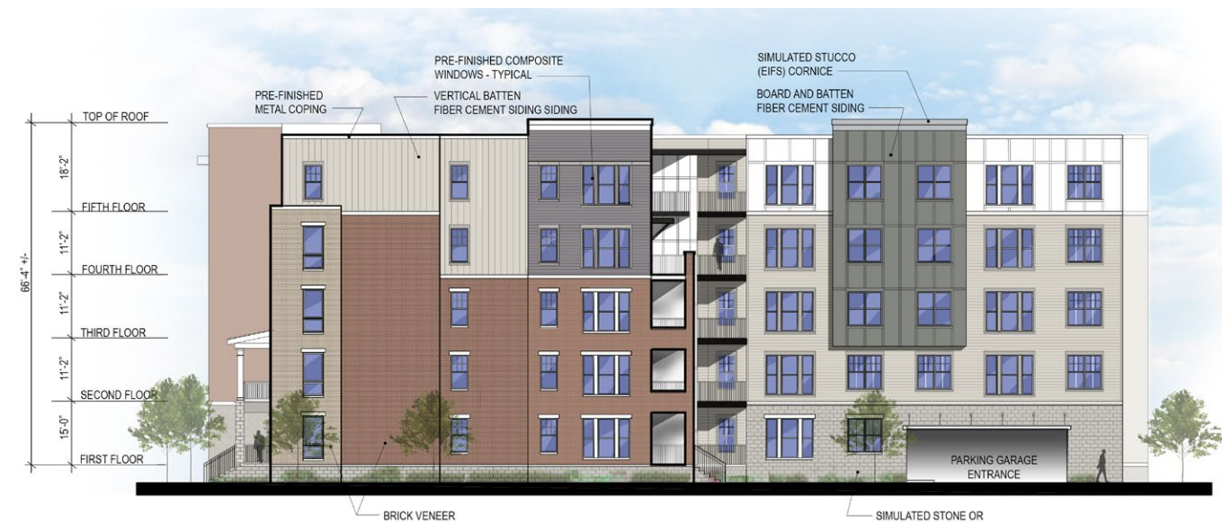
BUILDING 2 - ELEVATION D.2 (BLACK) - SOUTHEAST (NORTHWEST BROAD ENTRANCE) ELEVATION
