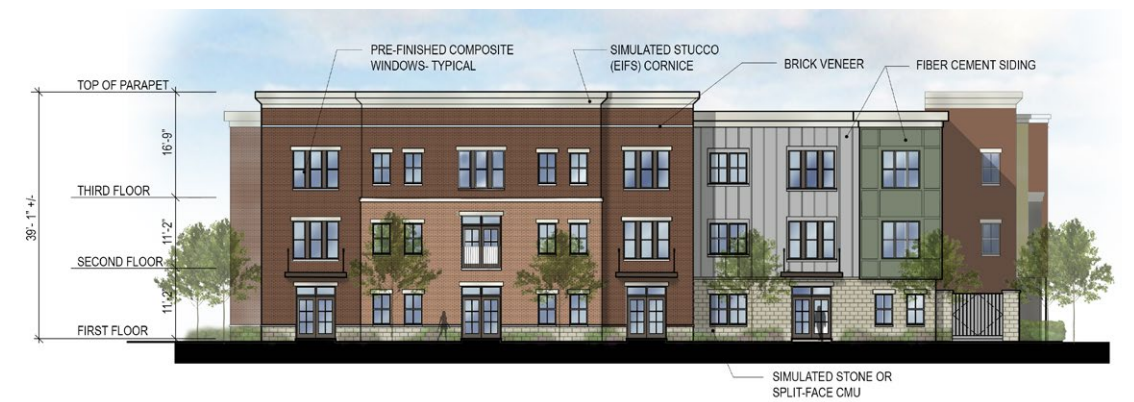
BUILDING 3 - ELEVATION C.3 (GREEN) - STATE STREET ELEVATION
