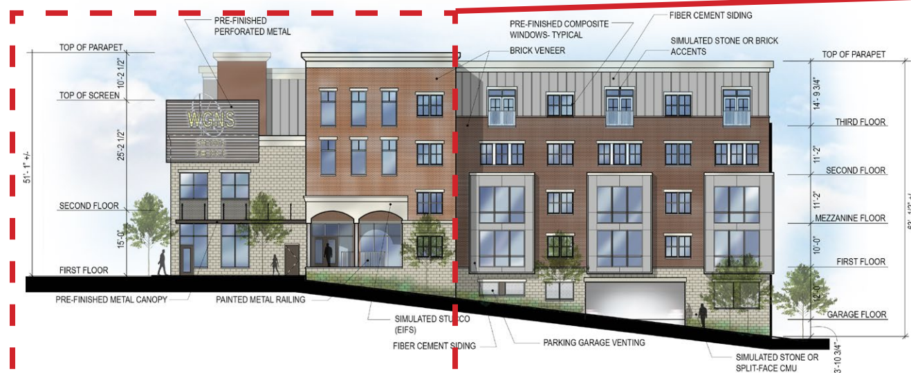
BUILDING 3 - ELEVATION A.3 (RED) - SOUTH CHURCH STREET ELEVATION
