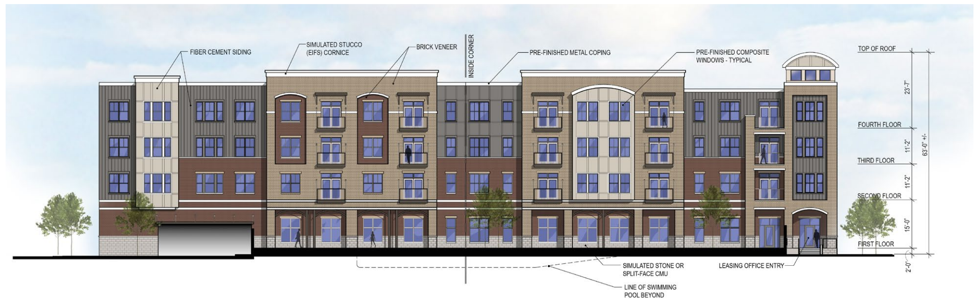
BUILDING 1 - ELEVATION B.1 (GREEN) - POOL SIDE AND LEASING OFFICE SIDE ELEVATION
