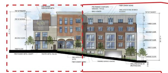
BUILDING 3 - ELEVATION A.3 (RED) - SOUTH CHURCH STREET ELEVATION
